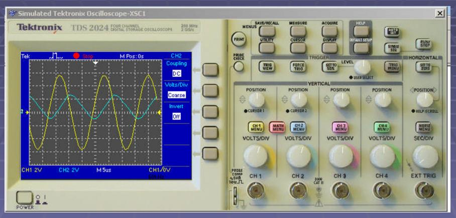
This is the scope showing the input (yellow) and the output (blue). The vertical sensitivities are the same for channel 1 & 2. The problem is that output voltage is definitely lower in amplitude than the input.
