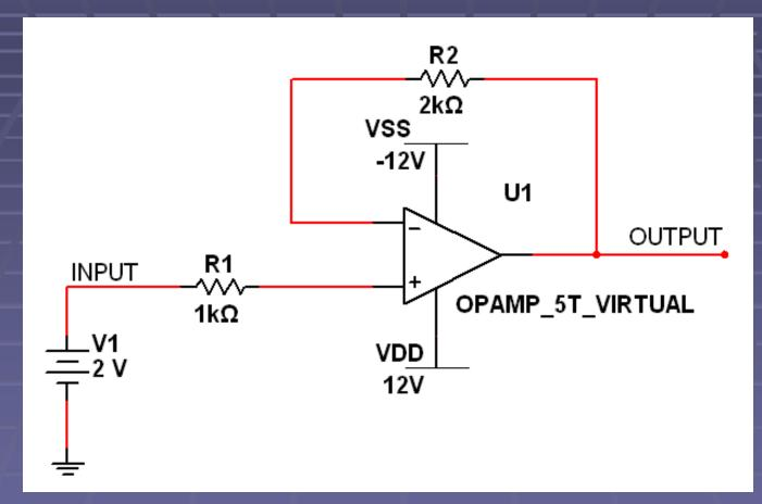
The power supplies are connected to the correct pins.
